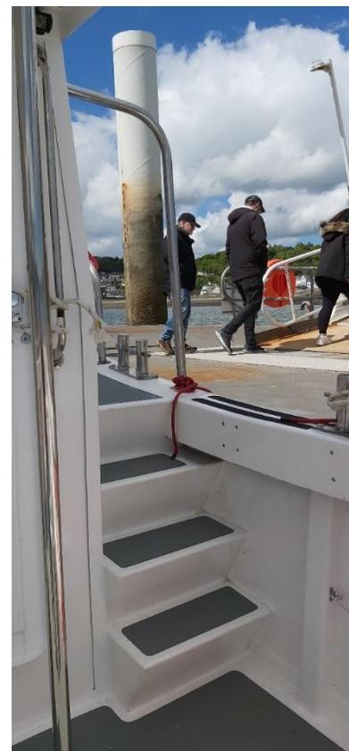
There is a gap between the vessel and the pontoon which passengers must step over. There are multiple handrails at different heights for passengers to use when boarding the vessel. There are then 4 steps down onto deck level, these steps are quite steep and may be best negotiated backwards like a ladder.
